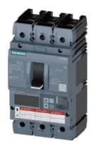
circuit breaker 3VA6 UL frame 150 breaking capacity class H 65kA @ 480 V 3-pole, line protection ETU556, LSI, In=40A overload protection Ir=16A ...40A short-circuit protection Isd=0.6..10x In, li=1.5..12x In N conductor protection opt. w. ext. CT; up to 160% ground-fault alarm message via EFB300 or COM nut keeper kit on both sides
