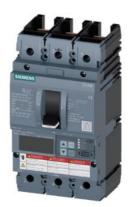
Circuit breaker 3VA6 UL Frame 150 breaking capacity class H 65kA @ 480V 3-pole, Line protection ETU556, LSI, In=40A overload protection, 100% rated Ir=16A...40A Short-circuit protection Isd=0.6..10x In, Ii=1.5..12x In N conductor protection optionally with external CT, up to 160% Ground-fault alarm message via EFB300 or COM without connection
