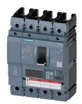
circuit breaker 3VA6 UL frame 150 breaking capacity class H 65kA @ 480V 4-pole, line protection ETU560, LSIG, In=40A overload protection Ir=16A...40A short-circuit protection Isd=0.6..10x In, Ii=1.5..12x In N conductor protection adjustable (OFF, up to 160%) ground-fault protection Ig=0.375...1 x In= tg=0.05-0.8s without connection
