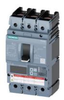
Circuit breaker 3VA6 UL Frame 150 breaking capacity class H 65kA @ 480 V 3-pole, Line protection ETU560, LSIG, In=40A overload protection, 100% rated Ir=16A ...40A Short-circuit protection Isd=0.6..10x In, Ii=1.5..12x In N conductor protection optionally with external CT; up to 160% Ground-fault protection Ig=0.375...1x In, tg=0.05-0.8s cable connection on both sides
