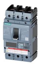
circuit breaker 3VA6 UL frame 150 breaking capacity class H 65kA @ 480 V 3-pole, line protection ETU560, LSIG, ln=40A overload protection lr=16A ...40A short-circuit protection lsd=0.6..10x ln, li=1.5..12x ln N conductor protection opt. w. ext. CT; up to 160% ground-fault protection lg=0.375...1x ln, tg=0.05-0.8s cable connection on both sides
