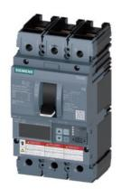
circuit breaker 3VA6 UL frame 150 breaking capacity class H 65kA @ 480 V 3-pole, line protection ETU560, LSIG, In=40A overload protection Ir=16A ...40A short-circuit protection Isd=0.6..10x In, Ii=1.5..12x In N conductor protection opt. w. ext. CT; up to 160% ground-fault protection Ig=0.375...1x In, tg=0.05-0.8s nut keeper kit on both sides
