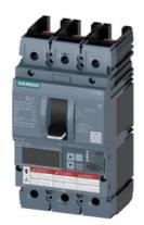
Circuit breaker 3VA6 UL Frame 150 breaking capacity class H 65kA @ 480V 3-pole, Line protection ETU560, LSIG, In=40A overload protection, 100% rated Ir=16A...40A Short-circuit protection Isd=0.6..10x In, Ii=1.5..12x In N conductor protection optionally with external CT, up to 160% Ground-fault protection Ig=0.375...1 x In, tg=0.05-0.8s without connection
