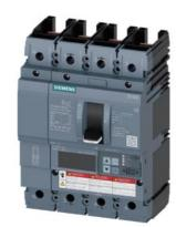
Circuit breaker 3VA6 UL Frame 150 breaking capacity class H 65kA @ 480V 4pole, Line protection ETU550, LSI, In=40A overload protection, 100% rated Ir=16A...40A Short-circuit protection Isd=0.6..10x In, Ii=1.5..12x In N conductor protection adjustable (OFF, up to 160%) without connection
