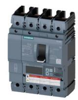
circuit breaker 3VA6 UL frame 150 breaking capacity class H 65kA @ 480V 4-pole, line protection ETU550, LSI, In=40A overload protection Ir=16A...40A short-circuit protection Isd=0.6..10x In, Ii=1.5..12x In N conductor protection adjustable (OFF, up to 160%) without connection
