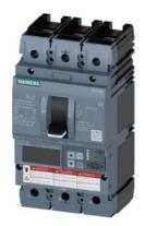
Circuit breaker 3VA6 UL Frame 150 breaking capacity class H 65kA @ 480 V 3-pole, Line protection ETU550, LSI, In=40A overload protection, 100% rated Ir=16A ...40A Short-circuit protection Isd=0.6..10x In, Ii=1.5..12x In N conductor protection optionally with external CT; up to 160% nut keeper kit on both sides
