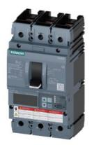
circuit breaker 3VA6 UL frame 150 breaking capacity class H 65kA @ 480 V 3-pole, line protection ETU550, LSI, In=40A overload protection Ir=16A ...40A short-circuit protection Isd=0.6..10x In, Ii=1.5..12x In N conductor protection opt. w. ext. CT; up to 160% nut keeper kit on both sides
