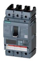
Circuit breaker 3VA6 UL Frame 150 breaking capacity class H 65kA @ 480V 3-pole, Line protection ETU550, LSI, In=40A overload protection, 100% rated Ir=16A...40A Short-circuit protection Isd=0.6..10x In, Ii=1.5..12x In N conductor protection optionally with external CT, up to 160% without connection
