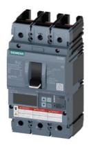
circuit breaker 3VA6 UL frame 150 breaking capacity class H 65kA @ 480V 3-pole, line protection ETU550, LSI, In=40A overload protection Ir=16A...40A short-circuit protection Isd=0.6..10x In, Ii=1.5..12x In N conductor protection optionally with external current transformer, up to 160% without connection
