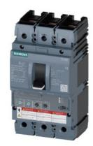
Circuit breaker 3VA6 UL Frame 150 breaking capacity class H 65kA @ 480 V 3-pole, Line protection ETU350, LSI, In=40A overload protection, 100% rated Ir=16A ...40A Short-circuit protection Isd=1.5... 10 x Ir, Ii=12 x In nut keeper kit on both sides
