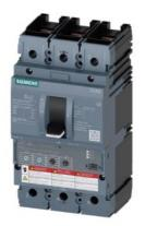
circuit breaker 3VA6 UL frame 150 breaking capacity class H 65kA @ 480 V 3-pole, line protection ETU350, LSI, In=40A overload protection Ir=16A ...40A short-circuit protection Isd=1.5... 10 x Ir, li=12 x In nut keeper kit on both sides
