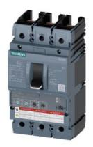
Circuit breaker 3VA6 UL Frame 150 breaking capacity class H 65kA @ 480V 3-pole, Line protection ETU350, LSI, In=40A overload protection, 100% rated Ir=16A...40A Short-circuit protection Isd=1.5...10 x Ir, Ii=12 x In without connection
