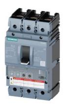
circuit breaker 3VA6 UL frame 150 breaking capacity class H 65kA @ 480 V 3-pole, line protection ETU330, LIG, ln=40A overload protection lr=16A ...40A short-circuit protection li=1.5...12 x ln ground-fault protection lg=0.375...1x ln, tg=0.1/0.3s cable connection on both sides
