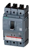
circuit breaker 3VA6 UL frame 150 breaking capacity class H 65kA @ 480V 3-pole, line protection ETU330, LIG, ln=40A overload protection lr=16A...40A short-circuit protection li=1.5...12 x ln ground-fault protection lg=0.375...1 x ln, tg=0.1/0.3s without connection
