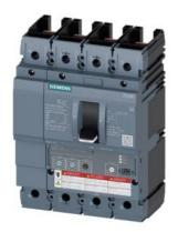
Circuit breaker 3VA6 UL Frame 150 breaking capacity class H 65kA @ 480V 4-pole, Line protection ETU320, LI, In=40A overload protection, 100% rated Ir=16A...40A Short-circuit protection Ii=1.5...12 x In N conductor protection adjustable (OFF, 100%) without connection
