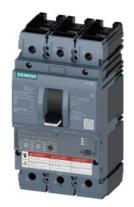
circuit breaker 3VA6 UL frame 150 breaking capacity class H 65kA @ 480 V 3-pole, line protection ETU320, LI, In=40A overload protection Ir=16A ...40A short-circuit protection Ii=1.5...12 x In nut keeper kit on both sides
