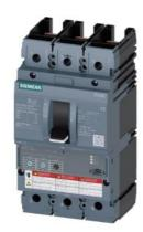
circuit breaker 3VA6 UL frame 150 breaking capacity class H 65kA @ 480V 3-pole, line protection ETU320, LI, In=40A overload protection Ir=16A...40A short-circuit protection Ii=1.5...12 x In without connection
