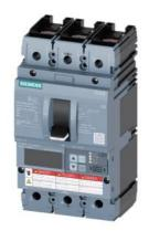
circuit breaker 3VA6 UL frame 150 breaking capacity class M 35kA @ 480 V 3-pole, line protection ETU856, LSI, In=40A overload protection Ir=16A ...40A short-circuit protection Isd=0.6..10x In, Ii=1.5..12x In N conductor protection opt. w. ext. CT; up to 160% ground-fault alarm message via EFB300 or COM cable connection on both sides
