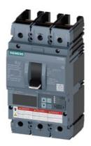
Circuit breaker 3VA6 UL Frame 150 breaking capacity class M 35kA @ 480V 3-pole, Line protection ETU856, LSI, In=40A overload protection, 100% rated Ir=16A...40A Short-circuit protection Isd=0.6..10x In, Ii=1.5..12x In N conductor protection optionally with external CT, up to 160% Ground-fault alarm message via EFB300 or COM without connection
