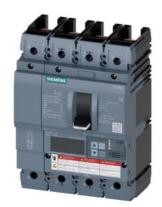
Circuit breaker 3VA6 UL Frame 150 breaking capacity class M 35kA @ 480V 4-pole, Line protection ETU860, LSIG, In=40A overload protection, 100% rated Ir=16A...40A Short-circuit protection Isd=0.6..10x In, Ii=1.5..12x In N conductor protection adjustable (OFF, up to 160%) Ground-fault protection Ig=0.375...1 x In=tg=0.05-0.8s without connection
