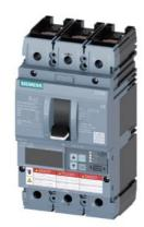
circuit breaker 3VA6 UL frame 150 breaking capacity class M 35kA @ 480 V 3-pole, line protection ETU860, LSIG, In=40A overload protection Ir=16A ...40A short-circuit protection Isd=0.6..10x In, Ii=1.5..12x In N conductor protection opt. w. ext. CT; up to 160% ground-fault protection Ig=0.375...1x In, tg=0.05-0.8s cable connection on both sides
