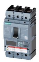
Circuit breaker 3VA6 UL Frame 150 breaking capacity class M 35kA @ 480 V 3-pole, Line protection ETU850, LSI, In=40A overload protection, 100% rated Ir=16A ...40A Short-circuit protection Isd=0.6..10x In, Ii=1.5..12x In N conductor protection optionally with external CT; up to 160% cable connection on both sides
