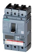
circuit breaker 3VA6 UL frame 150 breaking capacity class M 35kA @ 480 V 3-pole, line protection ETU850, LSI, In=40A overload protection Ir=16A ...40A short-circuit protection Isd=0.6..10x In, Ii=1.5..12x In N conductor protection opt. w. ext. CT; up to 160% cable connection on both sides
