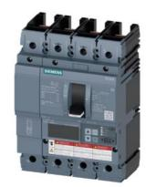
circuit breaker 3VA6 UL frame 150 breaking capacity class M 35kA @ 480V 4-pole, line protection ETU830, LIG, In=40A overload protection Ir=16A...40A short-circuit protection Ii=1.5...12 x In ground-fault protection Ig=0.375...1 x In, tg=0.05-0.8s without connection
