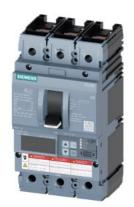
Circuit breaker 3VA6 UL Frame 150 breaking capacity class M 35kA @ 480 V 3-pole, Line protection ETU830, LIG, In=40A overload protection, 100% rated Ir=16A ...40A Short-circuit protection Ii=1.5...12 x In Ground-fault protection Ig=0.375...1x In, tg=0.05-0.8s cable connection on both sides
