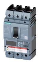
circuit breaker 3VA6 UL frame 150 breaking capacity class M 35kA @ 480 V 3-pole, line protection ETU830, LIG, ln=40A overload protection lr=16A ...40A short-circuit protection li=1.5...12 x ln ground-fault protection lg=0.375...1x ln, tg=0.05-0.8s cable connection on both sides
