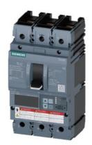
circuit breaker 3VA6 UL frame 150 breaking capacity class M 35kA @ 480 V 3-pole, line protection ETU830, LIG, ln=40A overload protection lr=16A ...40A short-circuit protection li=1.5...12 x ln ground-fault protection lg=0.375...1x ln, tg=0.05-0.8s nut keeper kit on both sides
