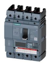
Circuit breaker 3VA6 UL Frame 150 breaking capacity class M 35kA @ 480V 4-pole, Line protection ETU820, LI, In=40A overload protection, 100% rated Ir=16A...40A Short-circuit protection li=1.5...12 x In without connection
