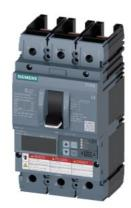
Circuit breaker 3VA6 UL Frame 150 breaking capacity class M 35kA @ 480V 3-pole, Line protection ETU820, LI, In=40A overload protection, 100% rated Ir=16A...40A Short-circuit protection Ii=1.5...12 x In without connection
