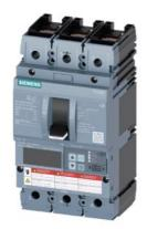
circuit breaker 3VA6 UL frame 150 breaking capacity class M 35kA @ 480 V 3-pole, line protection ETU556, LSI, In=40A overload protection Ir=16A ...40A short-circuit protection Isd=0.6..10x In, Ii=1.5..12x In N conductor protection opt. w. ext. CT; up to 160% ground-fault alarm message via EFB300 or COM cable connection on both sides
