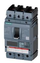
circuit breaker 3VA6 UL frame 150 breaking capacity class M 35kA @ 480 V 3-pole, line protection ETU556, LSI, In=40A overload protection Ir=16A ...40A shortcircuit protection Isd=0.6..10x In, Ii=1.5..12x In N conductor protection opt. w. ext. CT; up to 160% ground-fault alarm message via EFB300 or COM nut keeper kit on both sides
