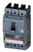
Circuit breaker 3VA6 UL Frame 150 breaking capacity class M 35kA @ 480V 3-pole, Line protection ETU556, LSI, In=40A overload protection, 100% rated Ir=16A...40A Short-circuit protection Isd=0.6..10x In, Ii=1.5..12x In N conductor protection optionally with external CT, up to 160% Ground-fault alarm message via EFB300 or COM without connection
