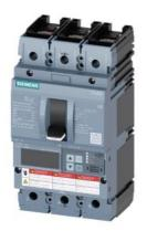
Circuit breaker 3VA6 UL Frame 150 breaking capacity class M 35kA @ 480 V 3-pole, Line protection ETU550, LSI, In=40A overload protection, 100% rated Ir=16A ...40A Short-circuit protection Isd=0.6..10x In, Ii=1.5..12x In N conductor protection optionally with external CT; up to 160% cable connection on both sides
