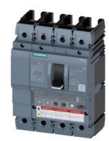
Circuit breaker 3VA6 UL Frame 150 breaking capacity class M 35kA @ 480V 4-pole, Line protection ETU350, LSI, In=40A overload protection, 100% rated Ir=16A...40A Short-circuit protection Isd=1.5...10 x Ir, Ii=12 x In N conductor protection adjustable (OFF, 100%) without connection
