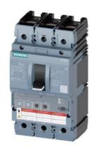
circuit breaker 3VA6 UL frame 150 breaking capacity class M 35kA @ 480 V 3-pole, line protection ETU350, LSI, In=40A overload protection Ir=16A ...40A short-circuit protection Isd=1.5... 10 x Ir, Ii=12 x In cable connection on both sides
