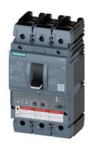
circuit breaker 3VA6 UL frame 150 breaking capacity class M 35kA @ 480 V 3-pole, line protection ETU350, LSI, In=40A overload protection Ir=16A ...40A short-circuit protection Isd=1.5... 10 x Ir, Ii=12 x In nut keeper kit on both sides
