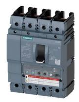
Circuit breaker 3VA6 UL Frame 150 breaking capacity class M 35kA @ 480V 4-pole, Line protection ETU330, LIG, ln=40A overload protection, 100% rated lr=16A...40A Short-circuit protection li=1.5...12 x ln N conductor protection adjustable (OFF, 100%) Ground-fault protection lg=0.375...1 x ln= tg=0.1/0.3s without connection
