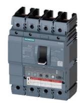
circuit breaker 3VA6 UL frame 150 breaking capacity class M 35kA @ 480V 4-pole, line protection ETU330, LIG, In=40A overload protection Ir=16A...40A short-circuit protection Ii=1.5...12 x In N conductor protection adjustable (OFF, 100%) ground-fault protection Ig=0.375...1 x In= tg=0.1/0.3s without connection
