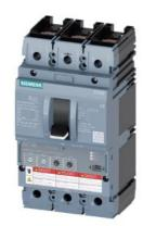
Circuit breaker 3VA6 UL Frame 150 breaking capacity class M 35kA @ 480 V 3-pole, Line protection ETU330, LIG, In=40A overload protection, 100% rated Ir=16A ...40A Short-circuit protection Ii=1.5...12 x In Ground-fault protection Ig=0.375...1x In, tg=0.1/0.3s cable connection on both sides
