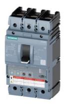
circuit breaker 3VA6 UL frame 150 breaking capacity class M 35kA @ 480 V 3-pole, line protection ETU330, LIG, ln=40A overload protection lr=16A ...40A short-circuit protection li=1.5...12 x ln ground-fault protection lg=0.375...1x ln, tg=0.1/0.3s cable connection on both sides
