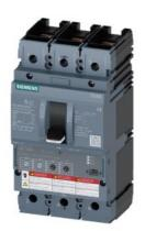
Circuit breaker 3VA6 UL Frame 150 breaking capacity class M 35kA @ 480 V 3-pole, Line protection ETU330, LIG, In=40A overload protection, 100% rated Ir=16A ...40A Short-circuit protection Ii=1.5...12 x In Ground-fault protection Ig=0.375...1x In, tg=0.1/0.3s nut keeper kit on both sides
