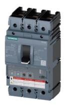
circuit breaker 3VA6 UL frame 150 breaking capacity class M 35kA @ 480 V 3-pole, line protection ETU330, LIG, ln=40A overload protection lr=16A ...40A short-circuit protection li=1.5...12 x ln ground-fault protection lg=0.375...1x ln, tg=0.1/0.3s nut keeper kit on both sides
