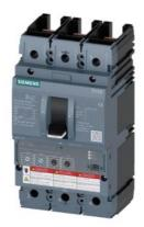
Circuit breaker 3VA6 UL Frame 150 breaking capacity class M 35kA @ 480V 3-pole, Line protection ETU330, LIG, In=40A overload protection, 100% rated Ir=16A...40A Short-circuit protection Ii=1.5...12 x In Ground-fault protection Ig=0.375...1 x In, tg=0.1/0.3s without connection
