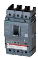
circuit breaker 3VA6 UL frame 150 breaking capacity class M 35kA @ 480V 3-pole, line protection ETU330, LIG, In=40A overload protection Ir=16A...40A short-circuit protection Ii=1.5...12 x In ground-fault protection Ig=0.375...1 x In, tg=0.1/0.3s without connection
