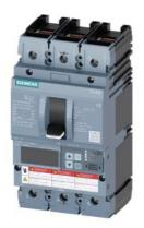
Circuit breaker 3VA6 UL Frame 150 breaking capacity class C 100kA @ 480 V 3-pole, Line protection ETU856, LSI, In=150A overload protection, 100% rated Ir=60A ...150A Short-circuit protection Isd=0.6..10x In, Ii=1.5..10x In N conductor protection optionally with external CT; up to 160% Ground-fault alarm message via EFB300 or COM cable connection on both sides
