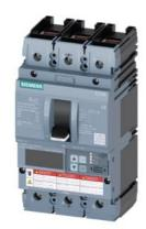
circuit breaker 3VA6 UL frame 150 breaking capacity class C 100kA @ 480 V 3pole, line protection ETU856, LSI, In=150A overload protection Ir=60A ...150A short-circuit protection Isd=0.6..10x In, Ii=1.5..10x In N conductor protection opt. w. ext. CT; up to 160% ground-fault alarm message via EFB300 or COM cable connection on both sides
